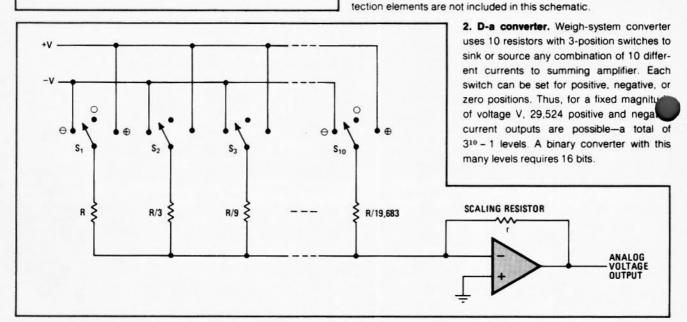
½(3<sup>n</sup>-1), whereas an n-bit binary system counts only to 2<sup>n</sup>-1. Therefore seven weights are approximately equivalent to 10 bits, and 10 weights are equivalent to 15 bits (or 16 bits with sign). This allows a dramatic compression of registers, counters, and wiring. Power consumption is also reduced, and speed is increased, especially if three-state devices are used.
